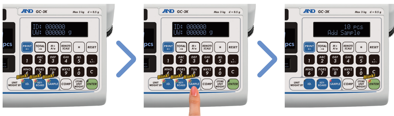
Example of selecting Sample Mode to set a unit weight
